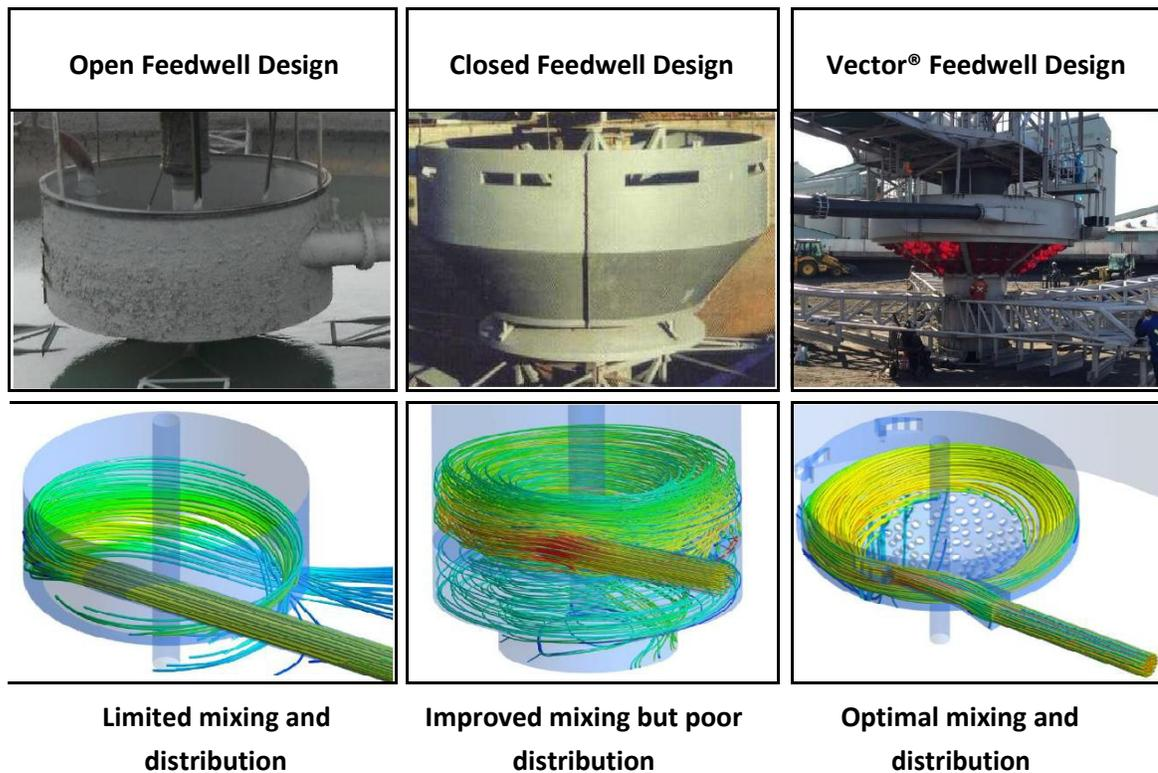
There became an apparent need to design a feed system that can operate in variable feed conditions, while still maintaining the correct amount of mixing and dilution that is required for
