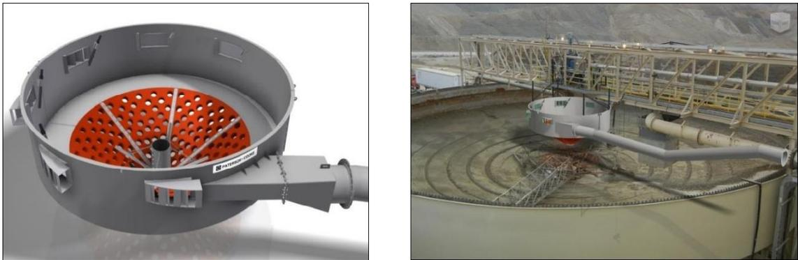
*Figure 8: Vector® feed system & 3D model and then overlaying on the existing equipment*
